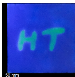
Figure 6. Representative lithographic pattern (HT) of B-SiC-dots/SiO 2 nanocomposite films (1.8 × 1.8 cm). NIR laser was used for patterning. UV light source at 375 nm was used to excite the film to induce PL.
